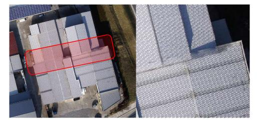
To eliminate the over-the-building image stitching we advise you to have the whole building on a single image. First, perform your mission at 80 m AGL, then manually trigger a few nadir images from a higher AGL (120 m above the object, for example) to get the whole object in one image.
