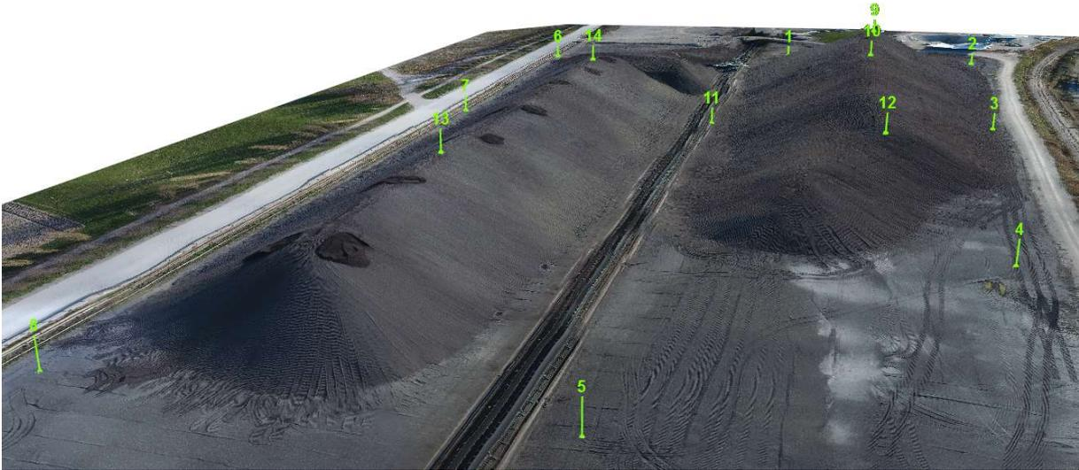
To achieve survey-grade accuracy, place your GCPs 50-100 m apart. Higher density of GCPs also means higher accuracy of end results.
